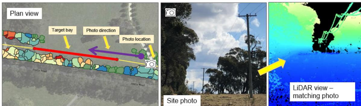
Figure 2: Ad-hoc checks looked at clearance, vegetated status, overstrike and hazard tree pattern matches – showing good general agreement.
