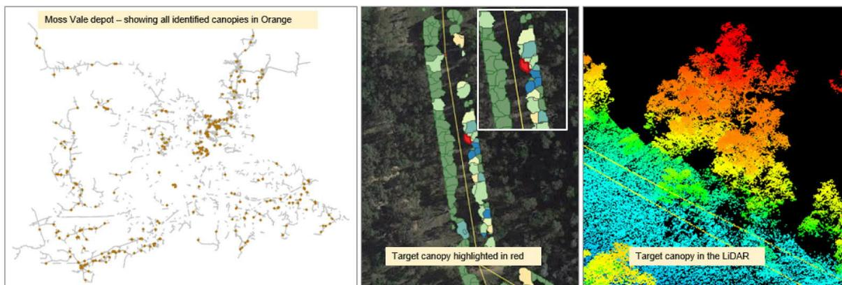
Figure 4: An example of a depot wide assessment of potential hazard trees showing a highly ranked as a tree in red, both in the GIS format and the lidar.
