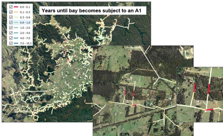
Figure 3: An example of outputs pertaining to the rate of growth of trees within individual spans
